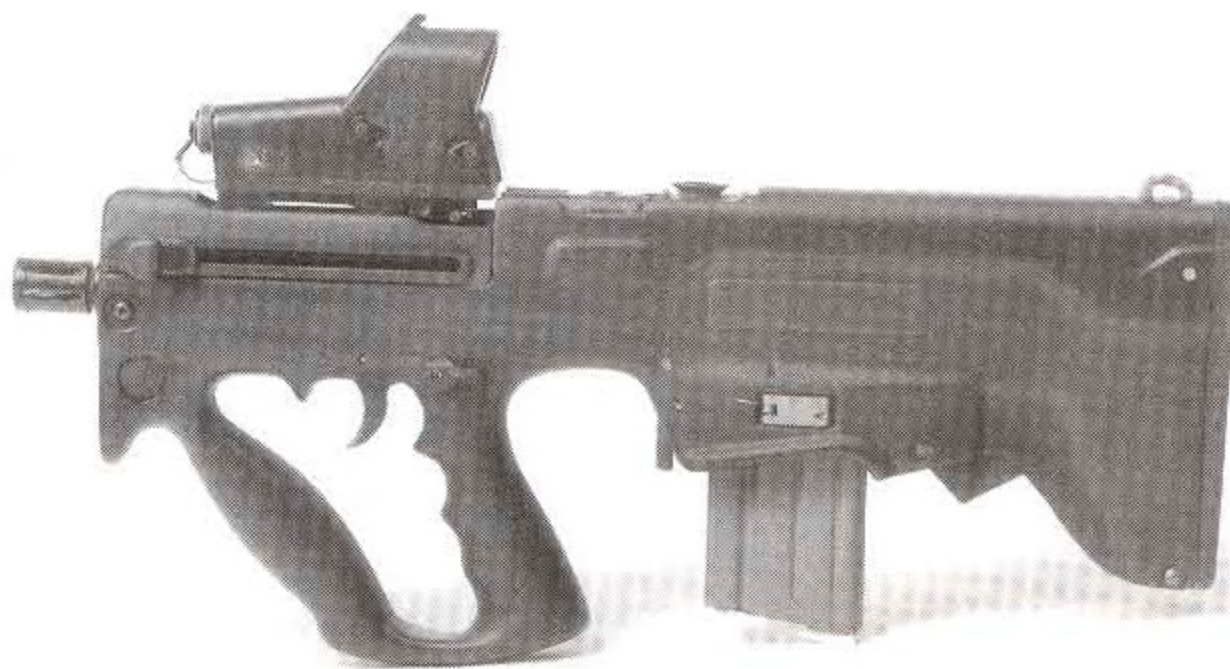
The TAR-21 Bullpup. (Right-side view). Heavy emphasis on the human engineering of the weapon is evident in the placement and design of the control levers. All were in easy reach when holding the weapon in the ready position. Magazine release, trigger, and slide release lever are designed for ambidextrous access. Charging (cocking) handle, selector lever, and ejection port can be quickly changed over for left-handed shooters. (IMI Photo)
