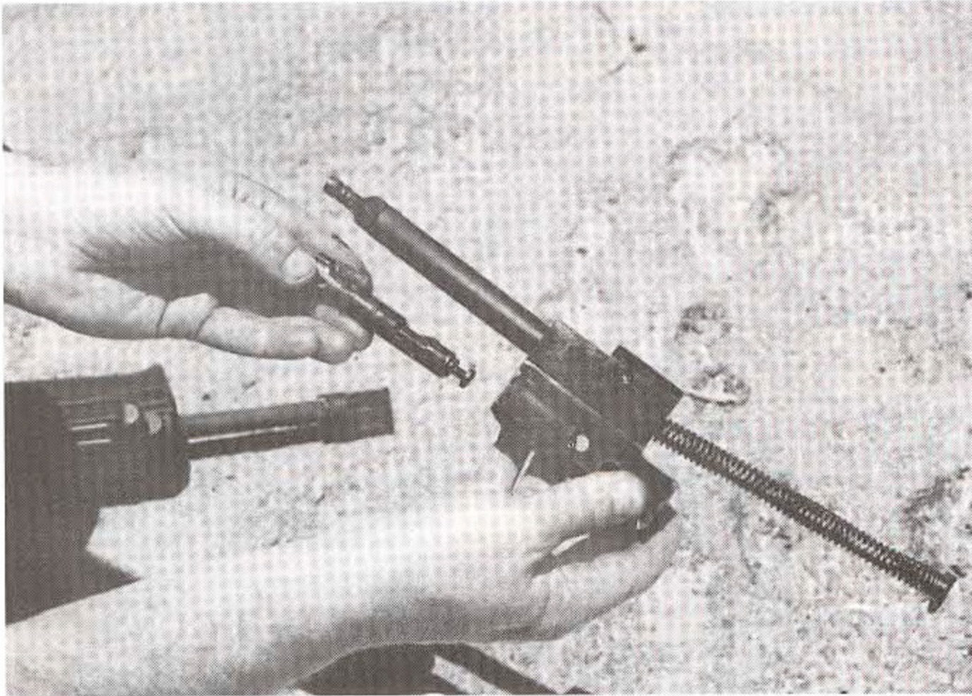
Bolt and firing pin being removed from carrier-group.
